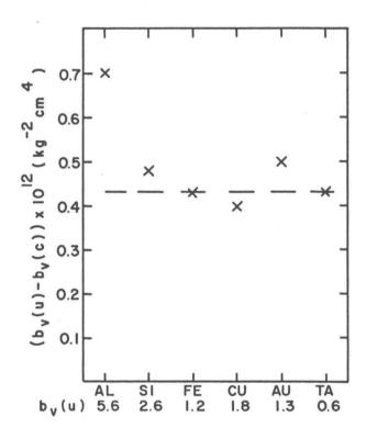
Fig. 3. Difference between ultrasonic and compression values of b for several incompressible elements. Dashed line represents the zero of ordinate corresponding to the correction proposed by Rotter and Smith (1).
